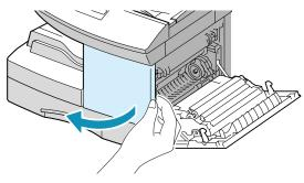
**2** Turn the cartridge locking lever upwards to unlock the toner cartridge, then pull the toner cartridge out.
